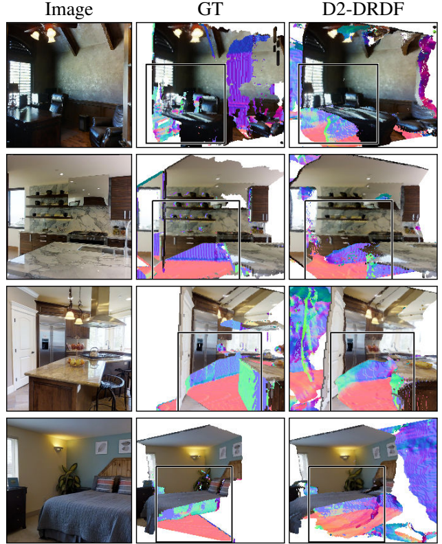
Figure 7. Novels Views Comparison between D2-DRDF and Ground Truth (GT) from novel views. Rows 1, 2 are from unseen images on Matterport3D [1] and 3,4 from Omnidata [11]. Our method trained with only RGBD data recovers occluded empty floors , kitchen cabinets (row 1) and sides of kitchen island (row 3).
